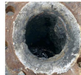
Hard water scale and corrosion before using Enmax CPRS
